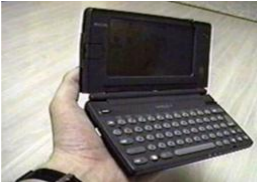
Figure 1. The Philips Velo 1 in hand. A full Windows CE handheld PC weighing under one pound, with web browsing, fax, voice memo, and Pocket Office applications.
