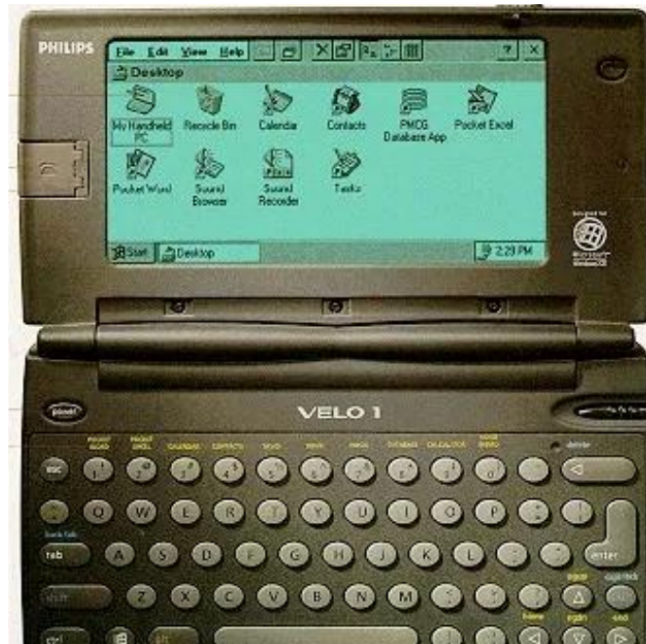
The Philips Velo 1: a full Windows CE handheld PC with Pocket Office, web browsing, fax, and voice memo capabilities.
