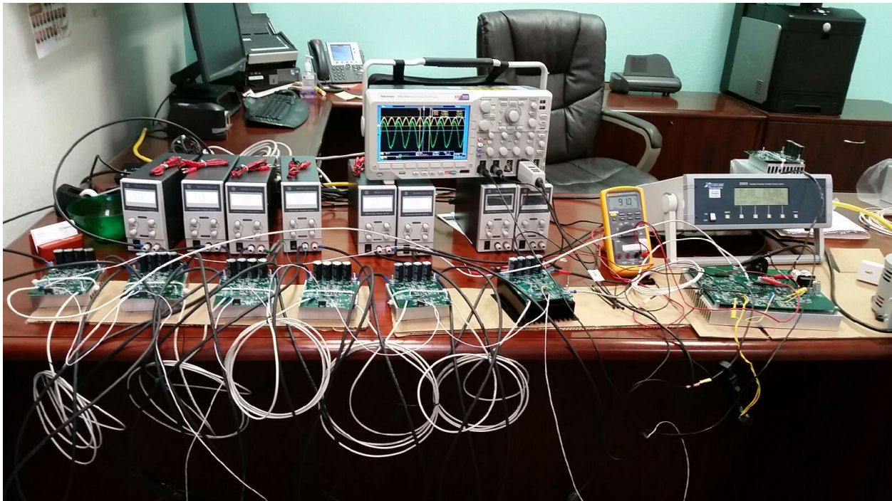
Figure 9. The system on the bench: multiple optimizer nodes wired as a simulated string, instrumented and driven, feeding the full chain that a real array would present. Proving the nodes add up in series was the milestone that turned a circuit into an architecture.
