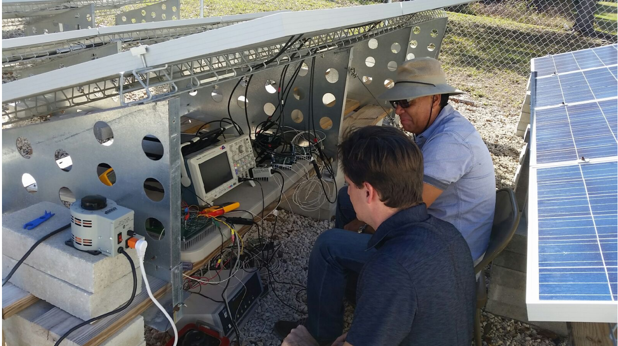
Figure 10. Field testing on a solar array — instrumenting the prototype outdoors, under load, into the grid. The step that separates a promising circuit from a product candidate.
