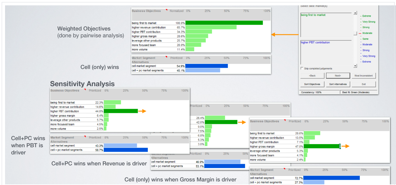
Figure 11. Pairwise comparison (right) produces weighted objectives; sensitivity analysis re-runs the market choice under different driving objectives. Toolkit example.
