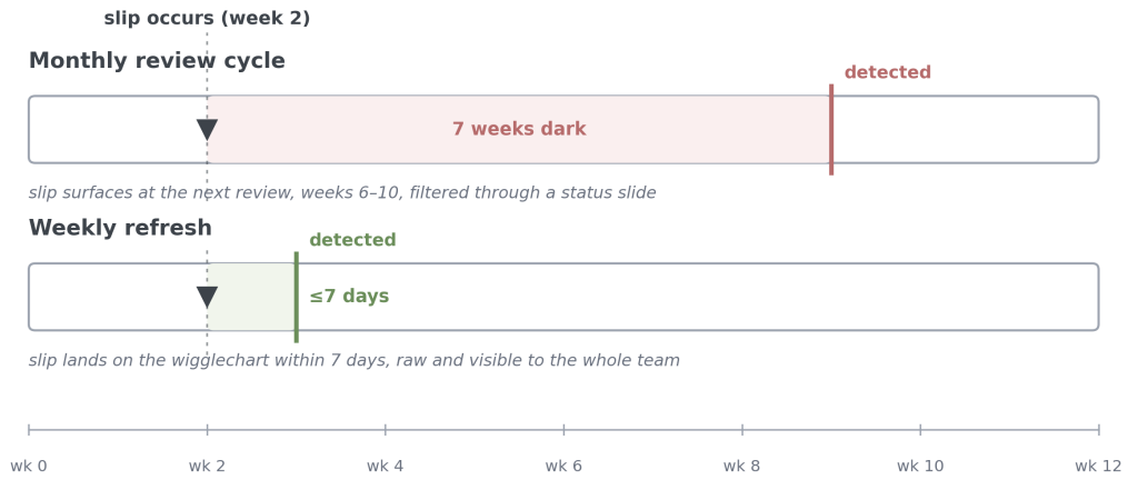
Figure 5. Feedback-loop compression. The same week-2 slip stays dark for weeks under a monthly review cycle; under a weekly refresh it is public within seven days, while corrective action is cheap.
