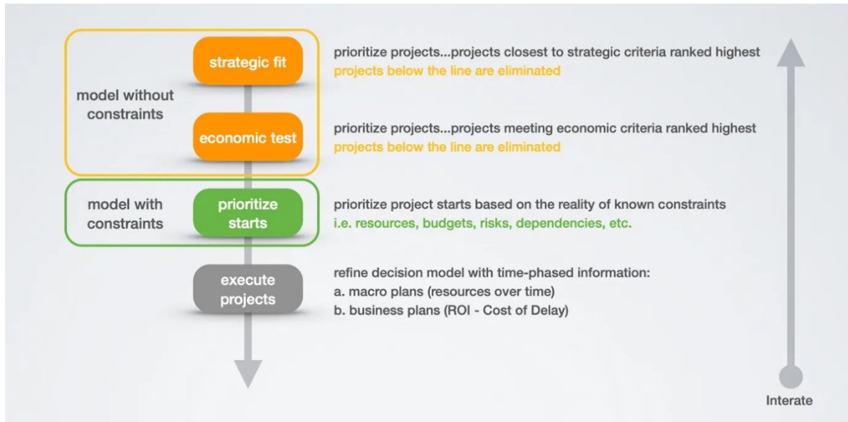
Figure 9. The portfolio modeling flow. The model without constraints ranks projects by strategic fit and economic test (projects below the line are eliminated). The model with constraints prioritizes starts against the reality of resources, budgets, risks, and dependencies. Execution refines the model with time-phased information; the loop iterates.
