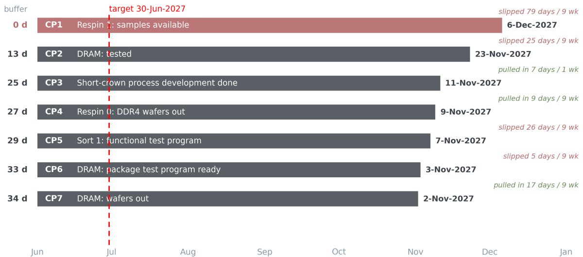
Figure 6. The onion on a live program: the top seven critical paths ranked by gap to target, with buffer held and nine-week trend for each. CP1 drives the date; CP2, slipping fastest, is the one to watch. Redrawn from a weekly fastProjectAI critical-path analysis [8].
