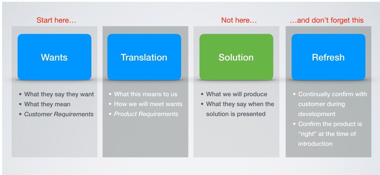
Figure 2. The four-step VOC loop. Fast teams enter at Wants and treat Refresh as a standing cadence. Teams that enter at Solution skip wants and translation and validate their own assumptions back to themselves [29].
