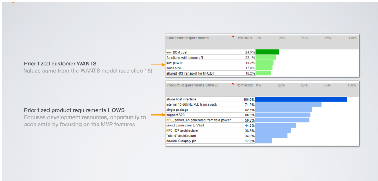
Figure 5. Product requirements (hows) ranked by their contribution to the prioritized customer wants. The shared host interface scores 100% because it serves four of the top five wants [29].
