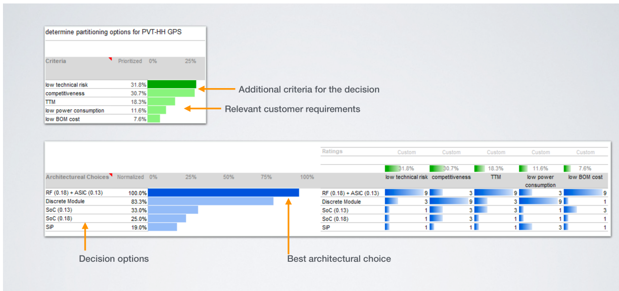
Figure 7. An architectural trade-off model combines customer wants (low power, low cost) with team criteria (technical risk, competitiveness, time-to-market). The combined ranking selects the architecture that best serves the weighted criteria [29].
