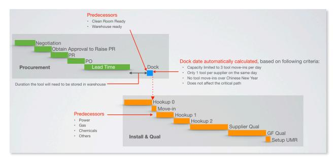
The main difference between the roll-up and roll-down, is dates from the FabX macro schedule are rolled-down whereas durations from the Module micro-schedules are rolled-up.
